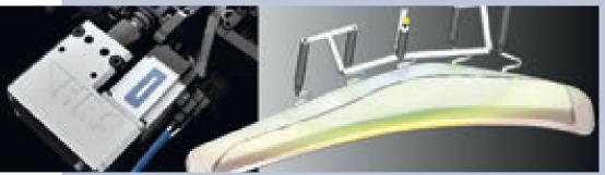
anced out. The cavity is filled with a uniform melt flow, as a result of which the surface of the moulded part does not have any optically relevant defects. The net result are high-quality, crystal-clear headlamp lenses that can be produced reliably and reproducibly - and with a thickness of only 1.8 mm instead of 2.5 mm and a weight of only 350 g instead of 450 g
