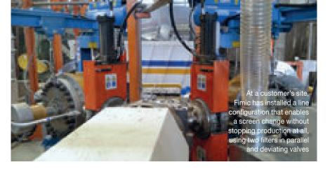
the backflushing feature, which enables filtration levels as low as 40 microns. Switching to this feature is a very simple operation to carry out. In fact, Fimic initial experience started with the backflushing function, while the scraping technology came later as further advancement. Unfortunately, backflushing has some limits, as it produces high losses during mesh cleaning (about twice as much when compared to the scraping technology) and it can operate only with low contamination levels.
