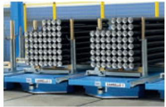
The Italian manufacturer IPM is also able to produce autonomous packaging plants, simultaneously managing pipes of different diameters and up to six different lengths, coming from four extrusion lines; it is able to manage and automatically pack up to 3,600 pipes per hour
