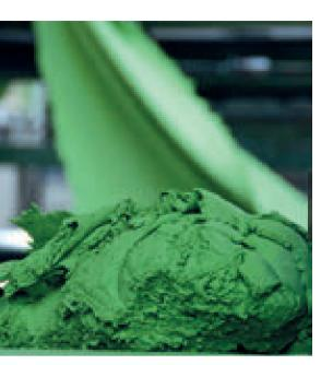
Instead of a filter die, Elastomers Union uses a gear pump to filter its polymers in order to obtain a less stressed product and avoid the breaking of the filters, a very common occurrence due to the high viscosity of the fluorinated polymer
