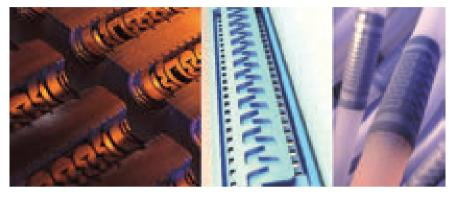
the production of round drip irrigation pipes with a production speed between 80 and 100 m per minute and an inserting capacity up to 400 drippers per minute, to produce pipes with diameter from 16 up to 20 mm.
