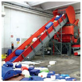
levels even with reduced diameter grilles (approximately 30 mm), resulting in very low management costs. Meanwhile, rotating-blade granulators are offered in capacities of up to 2.5 tons per hour for grinding mixed plastic waste produced in injection moulding, extrusion, blow moulding and thermoforming.
