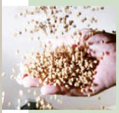
Biocomp granules, the innovative family of bioplastics developed by Microtec
