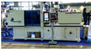
Fully electric Flower 100 (Euromap 100/322), with Dipre granulator (Main Tech) and TecnoMatic micro cnc handling equipment
