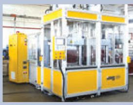
The special machine for BMC (Bulk Moulding Compound), used in the injection and compression moulding
