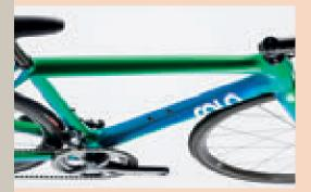
To achieve a slight flex, the Swedish bicycle manufacturer Rolo uses various carbon prepreg with tailor-made resin systems as well as a Kraibon inner layer in specific locations (photo: http://rolobikes.com)
